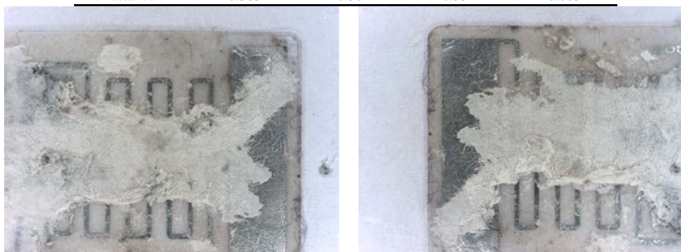
Figure 4. (a) Tag 2 after exposure to 50°C
