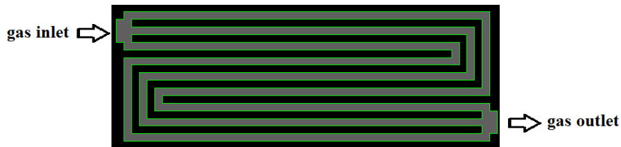
Figure 2. The bipolar plate flow channel pattern
