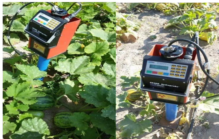
Figure 2. Measurements of soil moisture by a neutron probe under different dates
