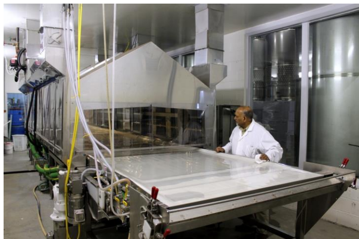
Figure 2. Industrial application of RW drying [5].
