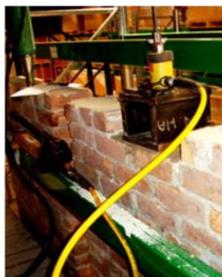
Figure 4. Post tensioning method
