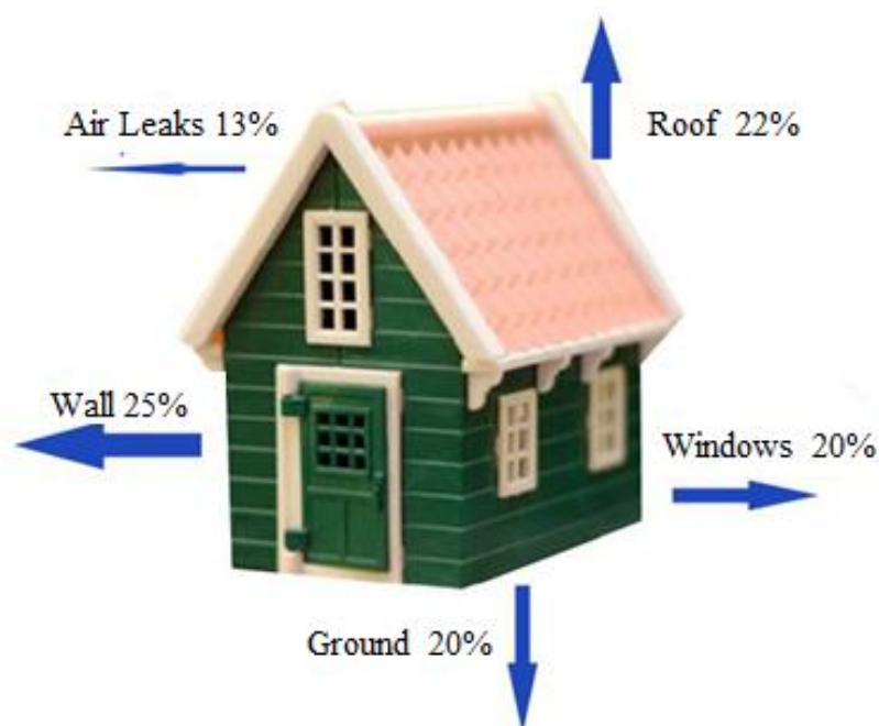
Figure 3 Average Heat Loss Ratios in Single Storey Buildings
